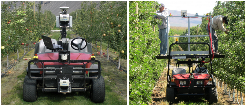
Fig. 1. (Left) Autonomous orchard vehicle “Laurel.” This experimental vehicle is equipped with encoders, laser rangefinder, cameras, and a differential GPS receiver for ground truth. (Right) “Cascade” in use by workers at Allan Bros. Orchards, in Prosser, WA, to thin green fruit. Time trials show that work on the top half of the trees, when conducted from the autonomous platform, can be more than twice as efficient than from ladders.
